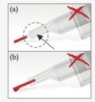
Avoid air bubbles and incomplete filling (a). Avoid sample on the outside of the capillary (b). Do not wipe off.
