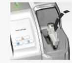
The lid opens automatically. Insert the Test Cartridge. The barcode should face left.
